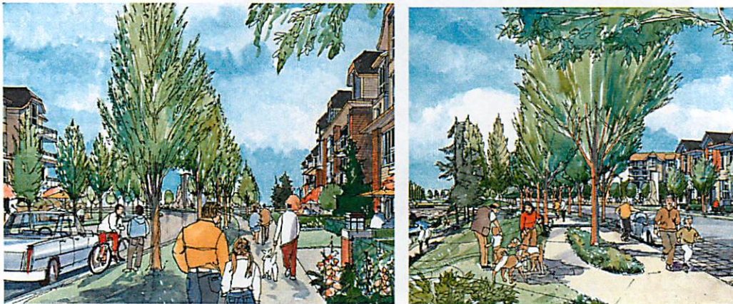
Fig. 17a and 17b: Developers shall be responsible for creating the street boulevard. A grass boulevard planted with trees provides a safe separation from the roadway and defines drop-off and parking areas along the street edge.
